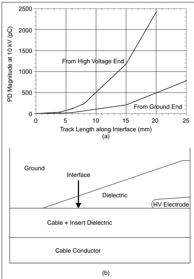
Fig. 3 Estimate of PD magnitude as a function of track length along the interface in a distribution joint. This is really a 3-D geometry, and various approximations were made to reduce the problem to 2-D. Consequently, these data must be considered approximate, but reasonably indicative.
