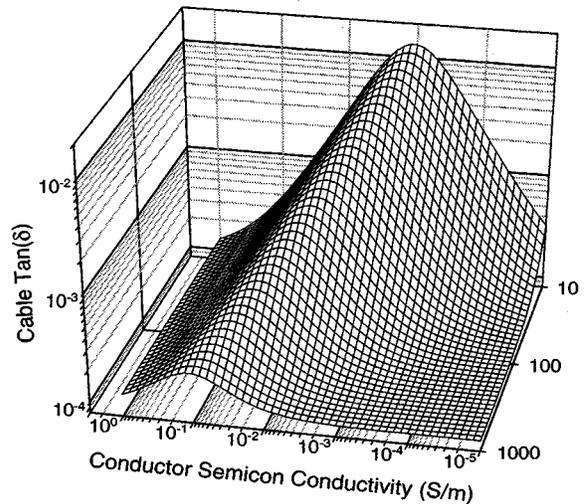
Fig. 4. Cable dielectric loss at 2 MHz as a function of conductor semicon conductivity and dielectric constant for a typical 15 kV class cable geometry. The characteristics of the ground shield semicon are such that they contribute little to the overall cable loss. The loss of the cable insulation is set to 0.001 which limits the lower bound of the cable loss to this value.
