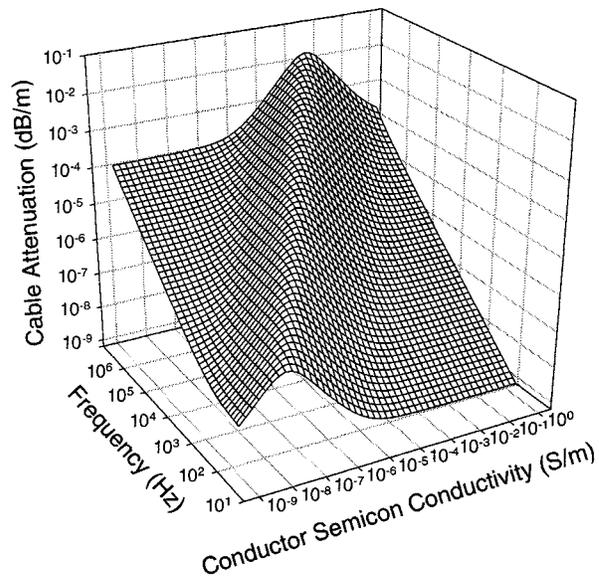
Fig. 5. Cable attenuation as a function of frequency and conductor semicon conductivity for a conductor semicon dielectric constant of ten. Note that the maximum loss is about 0.01 dB/m at 5 MHz and the optimum semicon conductivity. For a more typical semicon dielectric constant of 100, the attenuation would be reduced by about an order of magnitude.
