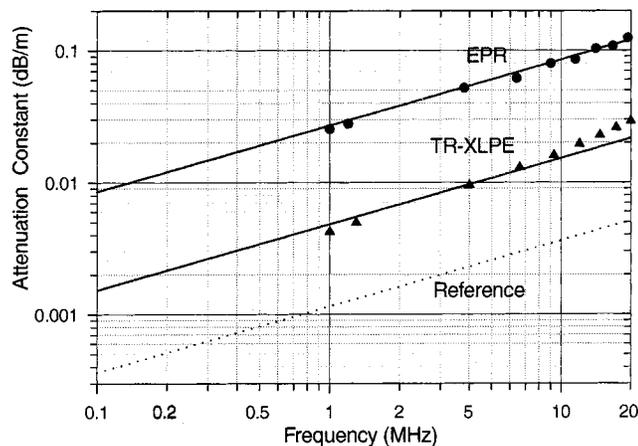
Fig. 6. High frequency attenuation of an EPR cable and a TR-XLPE cable. Symbols provide the data as measured with a high frequency impedance analyzer (HP4191A) while lines provide the calculated loss as implemented in the ATP-EMTP program. The attenuation of EPR cable is about an order of magnitude greater than that of TR-XLPE cable.
