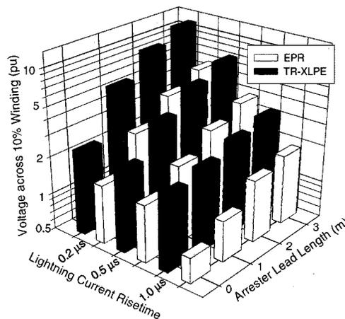
Fig. 12. Voltage in pu relative to peak line-to-ground voltage (10.78 kV) across the top 10% of the winding of Transformer 4 for a 40 kA lightning surge as a function of the lightning surge risetime, arrester lead length, and type of cable employed.
