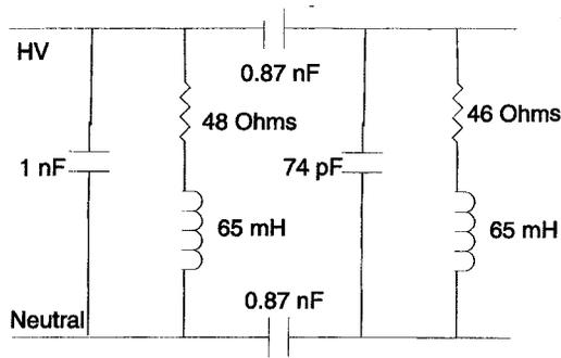
Fig. 3. High frequency electrical model for single-phase distribution transformer [2].
