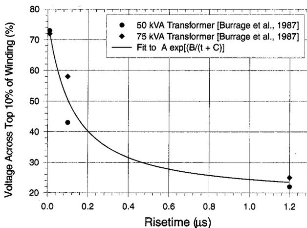
Fig. 11. Measured fraction of the voltage across the top 10% of a transformer winding for two different transformers [5] along with a curve fit to the data which is used in the present analysis.
