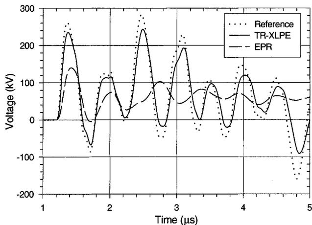
Fig. 10. Voltage across Transformer 4 (Fig. 2) for a 0.2  $\mu$ s risetime, 40 kA lightning surge with 3 m arrester lead length. The reflection from the open circuit causes a series of voltage peaks which are reduced in magnitude and damped out as a function of time by EPR cable in comparison with TR-XLPE cable.
