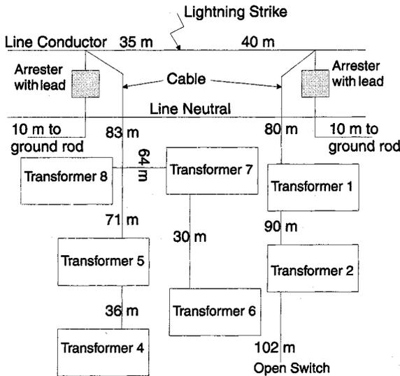
Fig. 2. Section of utility 13.2 kV distribution system which has been modeled. The transformers are modeled as shown in Fig. 3. The cable lengths are labeled in meters.
