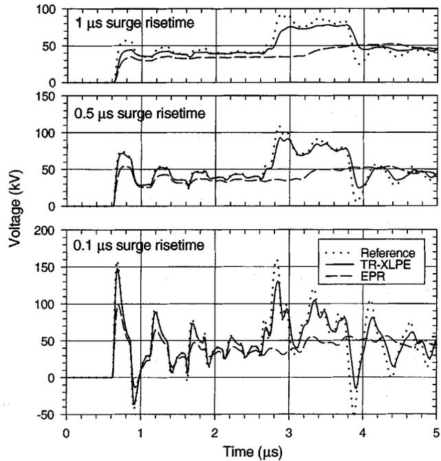
Fig. 8. Lightning-induced voltage at Transformer 1 (Fig. 2) for 40 kA lightning surge for various risetimes with an arrester lead length of 1 m. With decreasing current risetime, the transient overvoltage magnitude increases as does the  $dV/dt$  of the waveform. Again EPR cable reduces the initial peak voltage and damps the waveform rapidly.
