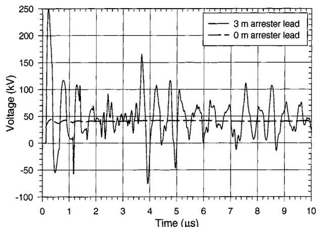
Fig. 1. Waveform across the right-branch cable input for the configuration shown in Fig. 2 for a 15 kV overhead line to cable connection at a riser pole. The lightning current was 40 kA with a risetime of 0.2  $\mu\text{s}$ . The arresters are gapless. Data are shown for 0 m and 3 m arrester lead lengths.
