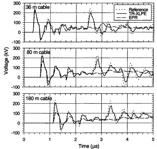
Fig. 9. Lightning-induced voltage at Transformer 1 for a  $0.1 \mu\text{s}$ , 40 kA lightning surge with 2 m arrester lead length and various cable lengths. Greater cable length decreases  $dV/dt$  of the initial transient. Again EPR cable damps the waveform rapidly to reduce the effect of reflections.
