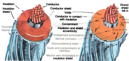
3. Although it is initially more costly, EPR cable insulation eliminates many of the causes of insulation failures that are found in cable insulation made of high-molecular-weight polyethylene (HMPE) or crosslinked-polyethylene (XLPE)
