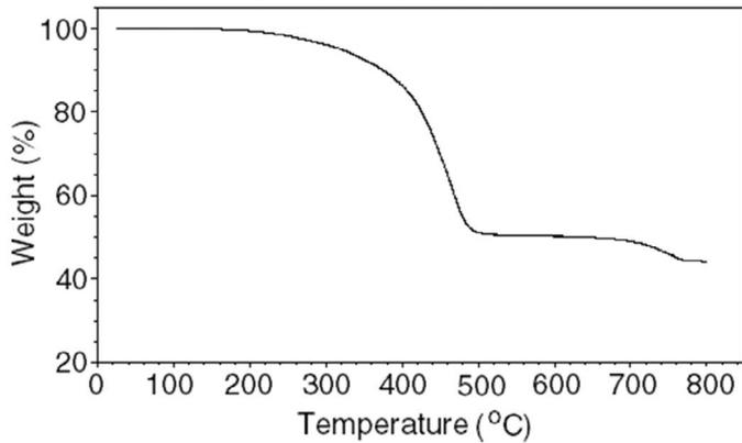
Figure 2. TGA thermogram for SBR cable dielectric. The heating rate is 20°C/min. and the purge gas is  $N_2$ .
