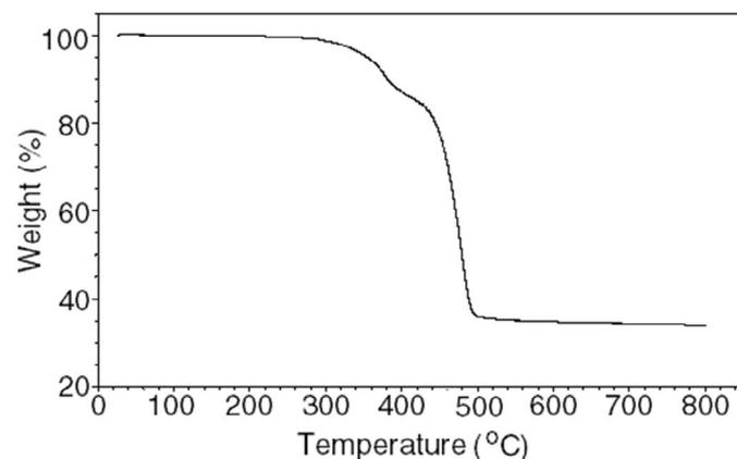
Figure 1. TGA thermogram for EPR cable dielectric. The heating rate is 20°C/min. and the purge gas is N<sub>2</sub>.
