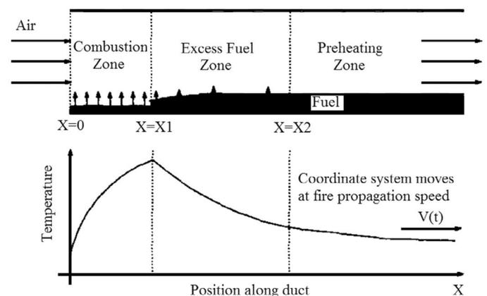
Figure 5. Model for one-dimensional duct fire propagation [19].
