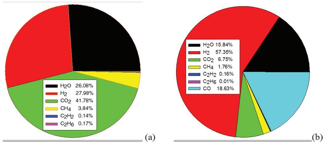
Figure 4. Composition of detectable gaseous products at 500°C (a) in air, and (b) in argon with 1% O<sub>2</sub>. In air, CO cannot be identified using an RGA because of interference from N<sub>2</sub>.
