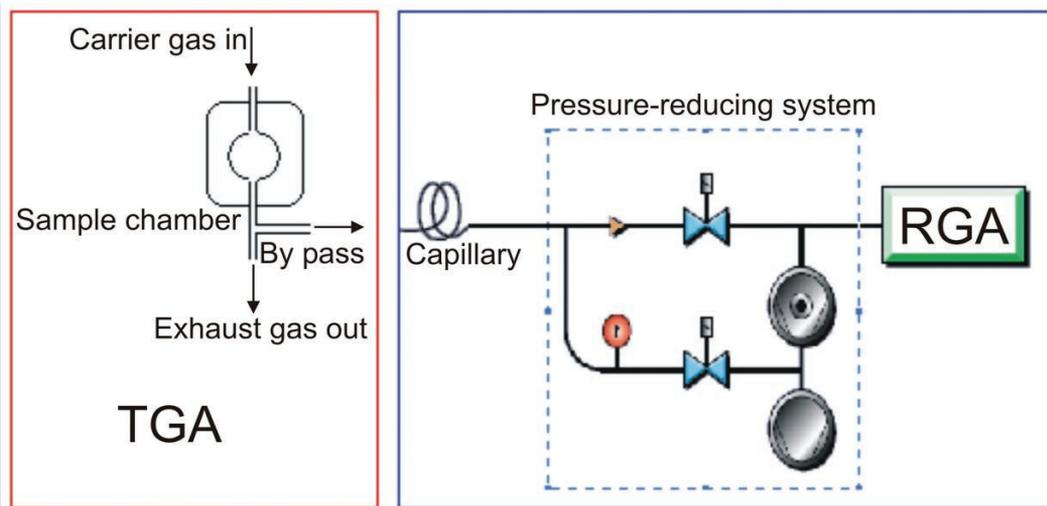
Figure 3. Schematic of evolved gas analysis system.
